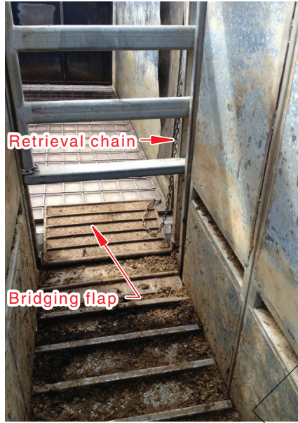
Figure B.3(I) — Accessible bridging flap retrieval chain at front of ramp and safety gate
