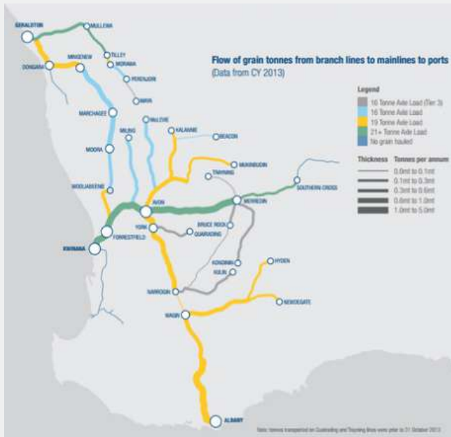
Figure 3.5 Western Australian grain rail lines by tier and volume of grain handled
