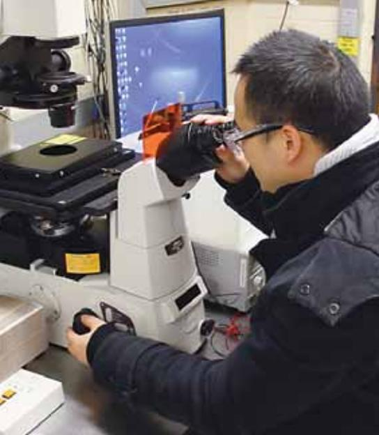
**RMIT University's Dr Jian Ou examines a membrane under a total internal reflection fluorescence microscope**
