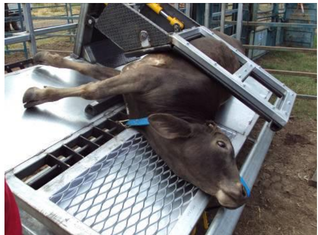
Figure 2 – Testing hydraulic Mark IV restraint box
